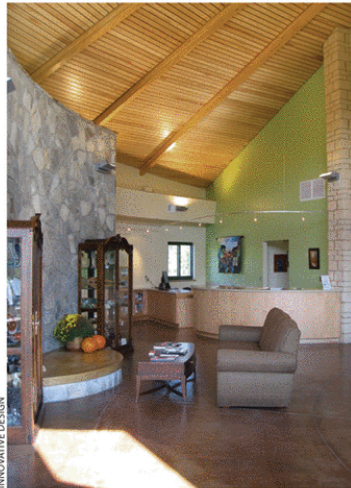
Daylighting provides two-thirds of the annual demand for lighting during daylight hours of the year.
